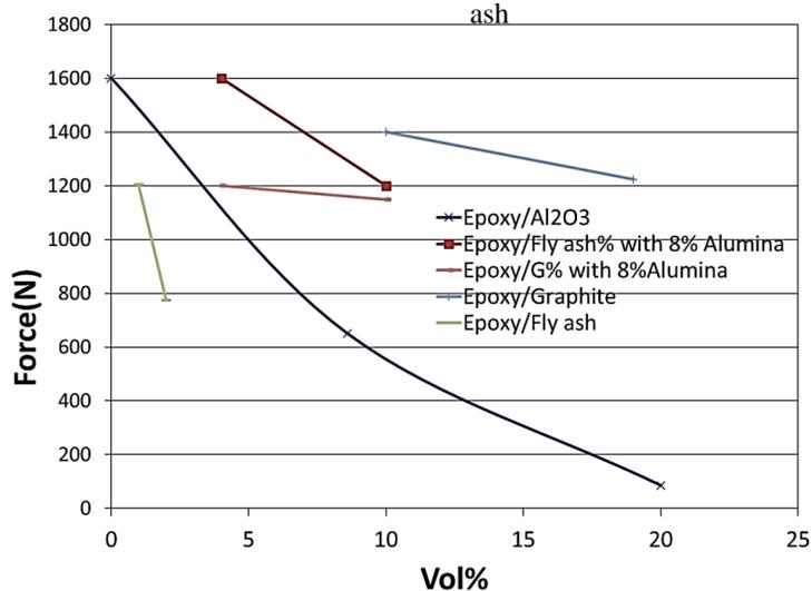
Fig. 2. The result of lap-shear test
